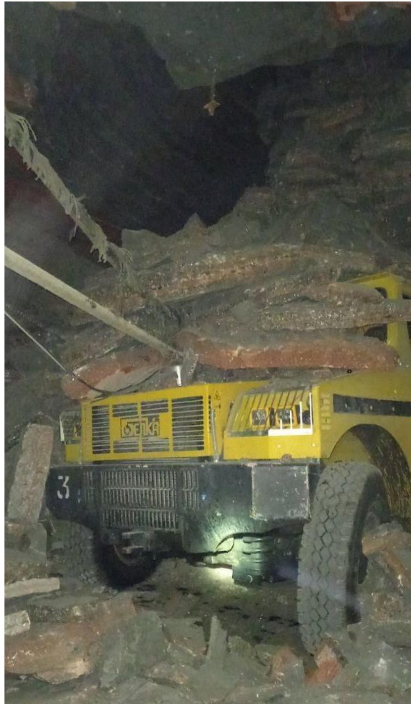
Figure 1. Rockburst, accompanied by gas release from camera K2 where the vehicle turns around (Mine 3, Second potash bed).
