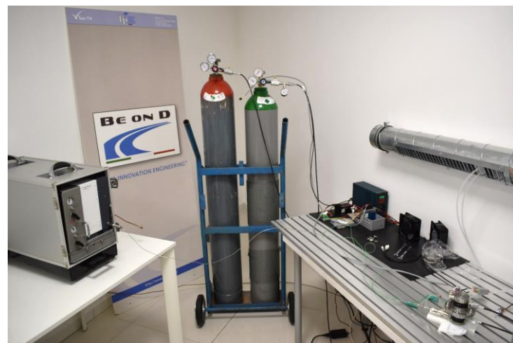
Figure 5. Permeability hydrogen test bench.
