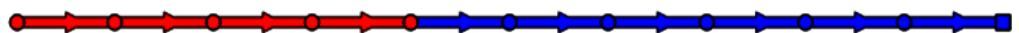
Figure 7. The net model of a straight microchannel. The red color shows the water distribution in the microchannel at the time of 2 s after the start of displacement.
