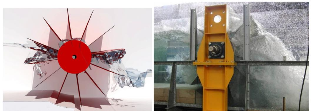
**Figure 23.** Lateral image of the instantaneous flow of water through the HPM for low discharge. **Left** image shows an instant of simulations with *caffa3d* for  $Q = 120$  L/s, while **right** image shows an instant of experimental tests for  $Q = 180$  L/s with the level downstream of the wheel 200 mm below the edge of the hub [38].
