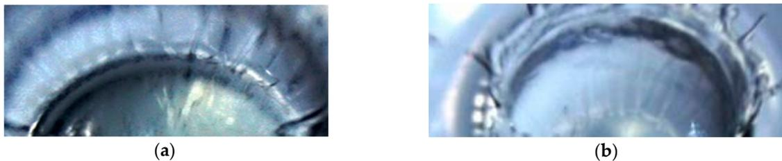
**Figure 15.** Enlarged images of the contact domain boundary of a merging saturated iron sulfate solution drop with water (parts of Figure 13). (a) fast jets forming linear structure on the cavity surface; (b) traces of jets—ligaments on the bottom of the cavity.
