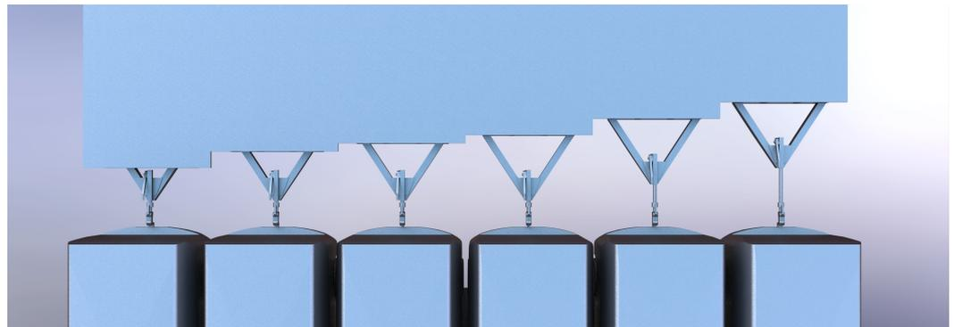
**Figure 18.** Image of the different drawbar lengths used in the drawbar length tests.
