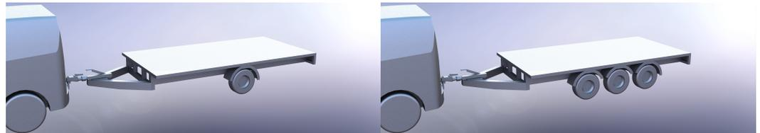
Figure 15. Images of the single- and triple-axle FBT1 configurations.
