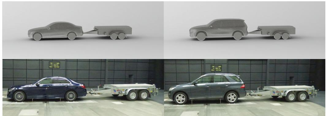
**Figure 1.** Image showing the simulated sedan and SUV geometry against that used in the wind tunnel test [4].
