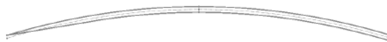
Figure 2. Cambered Plate, 0.05c of f (at x_c = 0.5c ), 0.01c thickness, with a 0.2c beveled bottom corner of the leading edge (LE).
