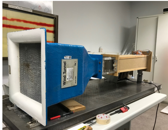
Figure 5. Main view of the low speed wind tunnel.
