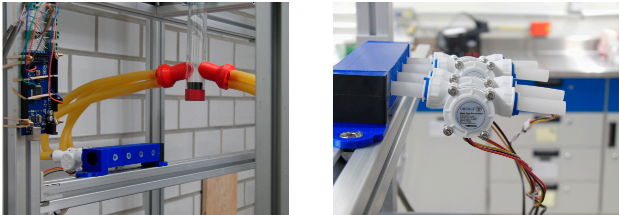
Figure 13. Experimental rig employed for measuring the volumetric flow at each quadrant and four digital rotational flow meters mounted on a horizontal hub.
