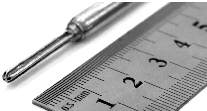
Figure 2. Multi-hole pressure probe.
