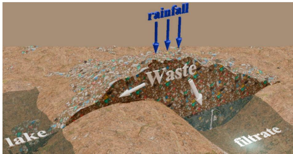
**Figure 1.** Scheme of accumulation of leachate in the area of lowering of the landfill of municipal solid waste. Designations: lake—landfill leachate pond, leachate—landfill leachate, waste—MSW body.
