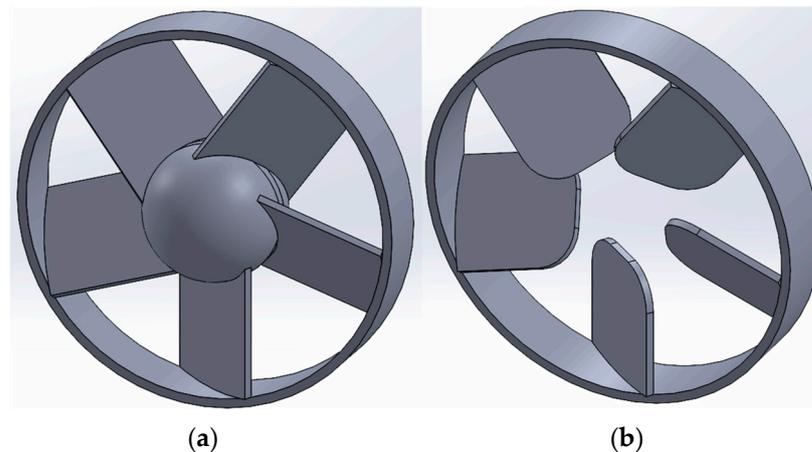
**Figure 5.** (a) Impeller with hub. (b) Hubless impeller. 5 simple (plain) blades were used. The device is driven from the side, hence the name “rim-driven thruster” (RDT). Diameter = 50 mm.
