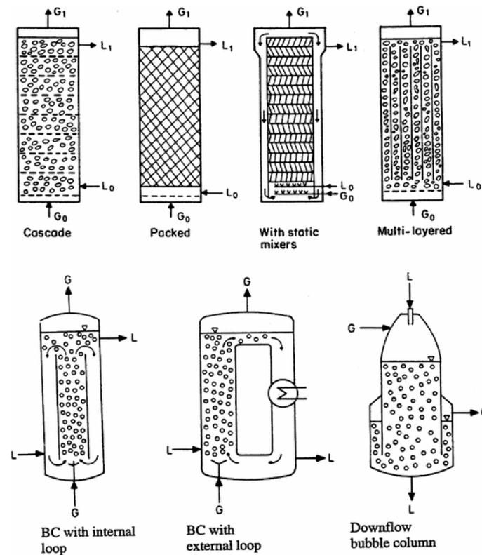
**Figure 2.** Different embodiments of bubble column reactors (BC). The BC with an external loop gives a homogeneous residence time distribution. Mass transfer is enhanced when an additional pump is deployed, which is how the loop reactor was developed. Source: [19] (reproduced with permission).
