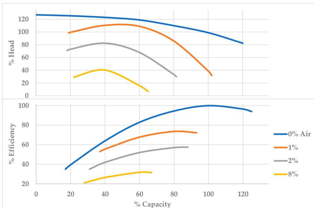
**Figure 1.** Schematic example for a set of pump curves as a function of gas fraction. Redrawn from [17].
