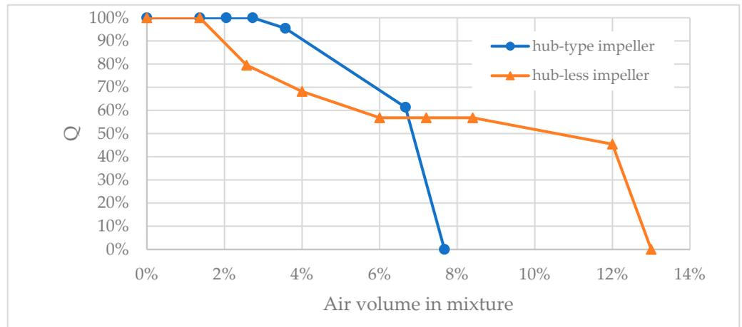
**Figure 6.** Total flow rate as function of air content in the fluid without guiding vanes. Impeller with hub (blue, circle) and hubless (orange, triangle). Configuration without guide vanes. The hubless setup can pump 5% more air fraction than the other one. Q = flow rate.
