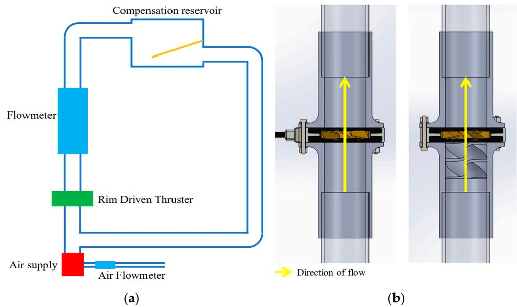
**Figure 4.** Experimental setup with details on static guide vanes. (a) Schematic illustration of the experimental setup. Total pipe length 6 m, flow rate clockwise. (b) The adapter without guide vanes is on the left and with guide vanes is on the right. Guide vanes provide a swirl, pushing the gas phase to the center of the RDT, increasing its performance.
