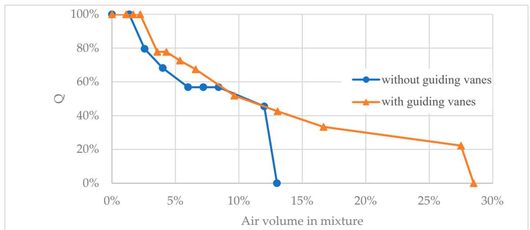
**Figure 8.** Total flow rate as function of air content in the fluid with hub-type impeller and direct comparison of the setups with guide vanes (orange line with triangles) and without guide vanes (blue with circles).
