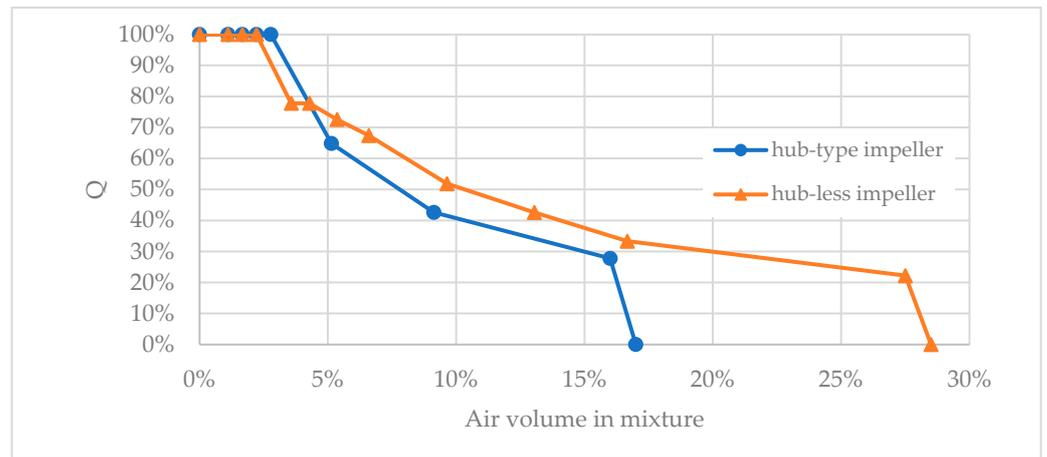
**Figure 7.** Total flow rate as function of air content in the fluid with guiding vanes. Impeller with hub (blue, circle) and hubless (orange, triangle). Configuration with guide vanes below the upwards-pumping RDT.
