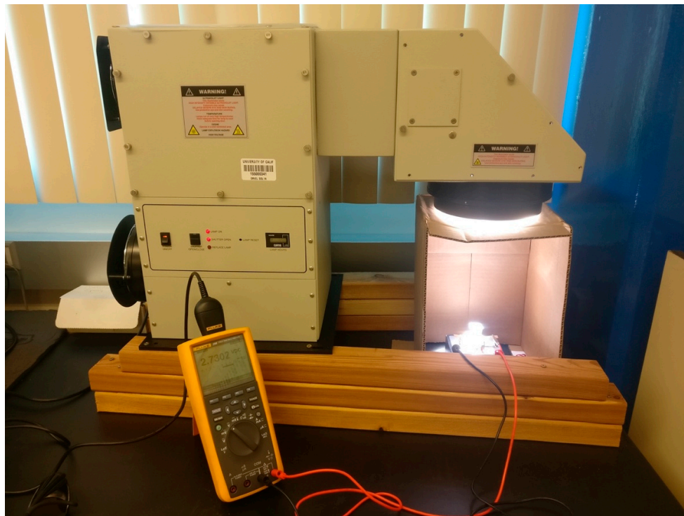
Figure S2. Actual experimental setup working at 70 suns illumination with multi-meter recording the open-circuit voltage.
