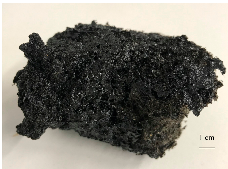
Figure 1. Picture of foamy PFA obtained from Zn-activated polymerization of FA at 80 °C.
