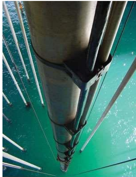
Figure 17. Composite drilling riser for offshore oil drilling: 15 m long, 59 cm inside diameter, 315 bar pressure; manufactured for Norske Conoco A/S and other oil companies (reprinted with permission from Ref. [1]).
