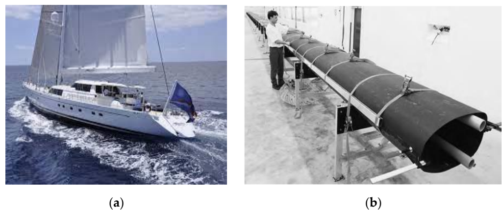
Figure 15. (a) Hyperion 2 yacht and (b) Hyperion 2 yacht mast with 59 m length fabricated from CFRP (adapted with permission from Refs. [36,55]).
