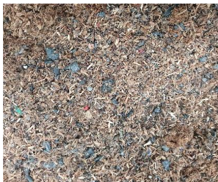
Figure 1. Mixture of WIEC and WLB used for the carbonization tests on a pilot scale.
