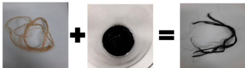
Figure 1. Schematic of the process of coating curauá fibers with MWCNTs.
