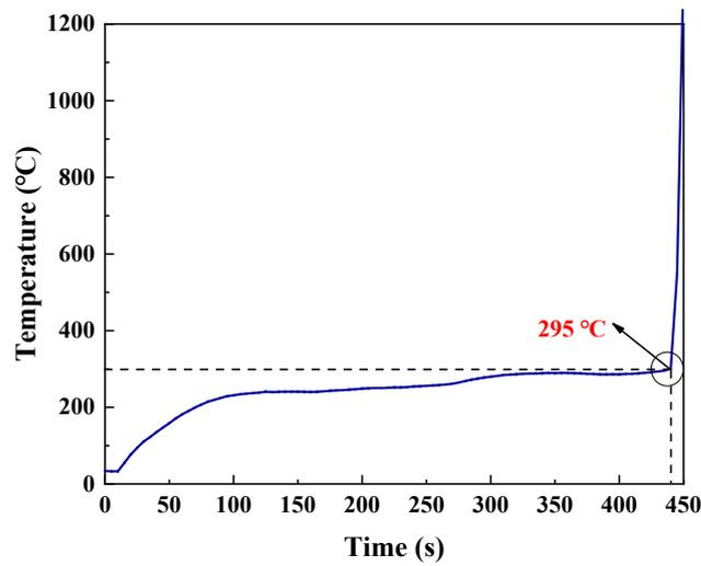
Figure 3. Temperatures of corn straw particles at 200 W.
