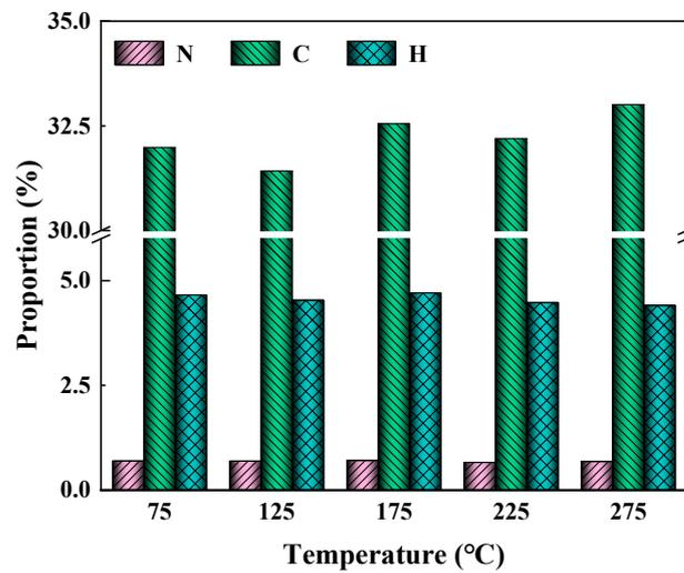
Figure 4. Proportions of C, H, and N elements at different temperatures (10 min).
