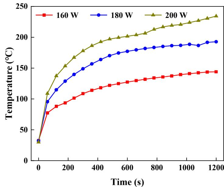
**Figure 6.** Temperatures of corn straw particles at different microwave powers.
