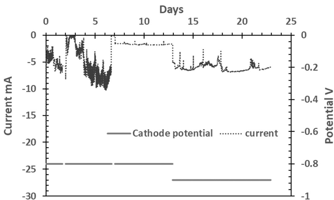
Figure S1: Profiles of cathode potentials and electric current in CuBP2 MES.
