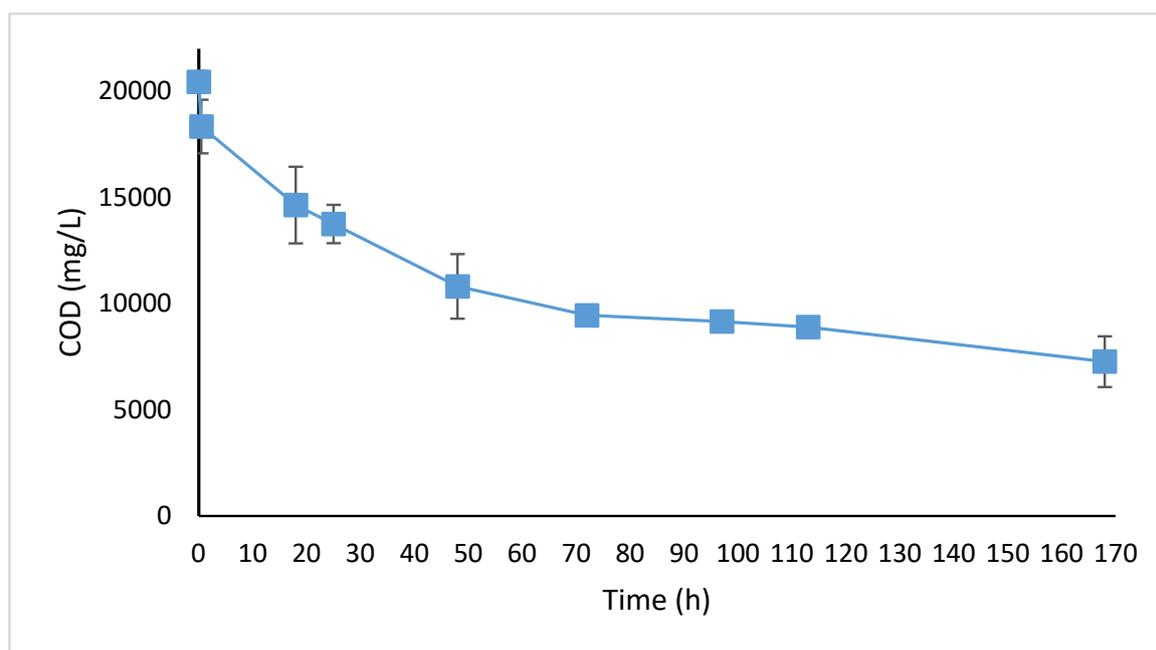
**Figure 6.** COD degradation in Stage I operational cycles with 2.4 g/L  $\text{NH}_4\text{Cl}$  addition.
