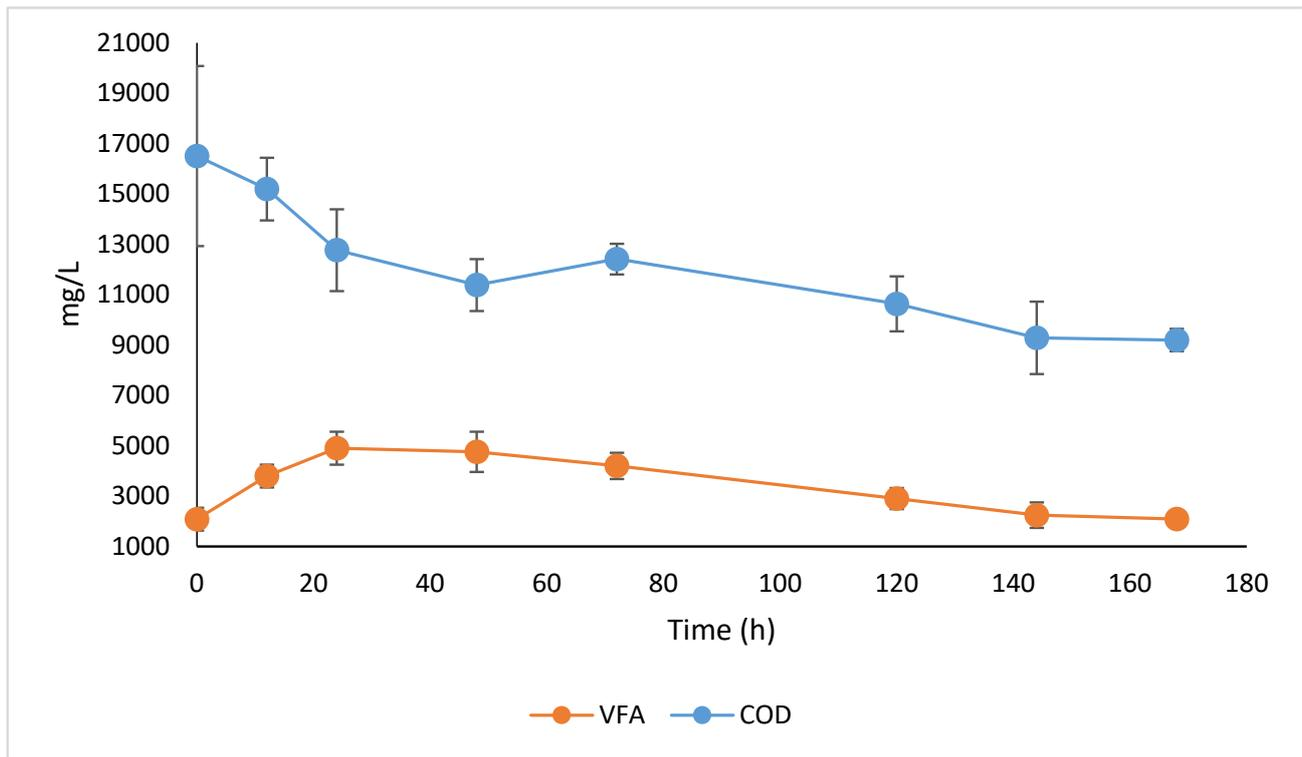
**Figure 4.** Degradation of VFA and COD in the operational cycles of increasing reaction time to 168 h.
