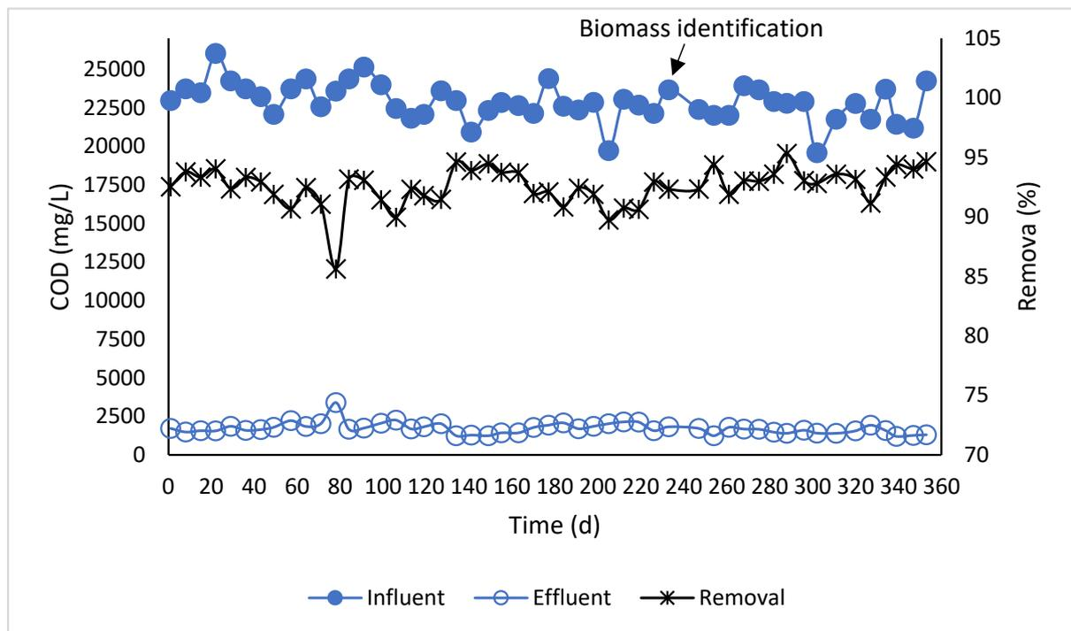
**Figure 8.** Behavior of COD with optimal conditions (RT = 168 h, initial concentration of vinasse = 60%, C/N ratio = 100/1.9).
