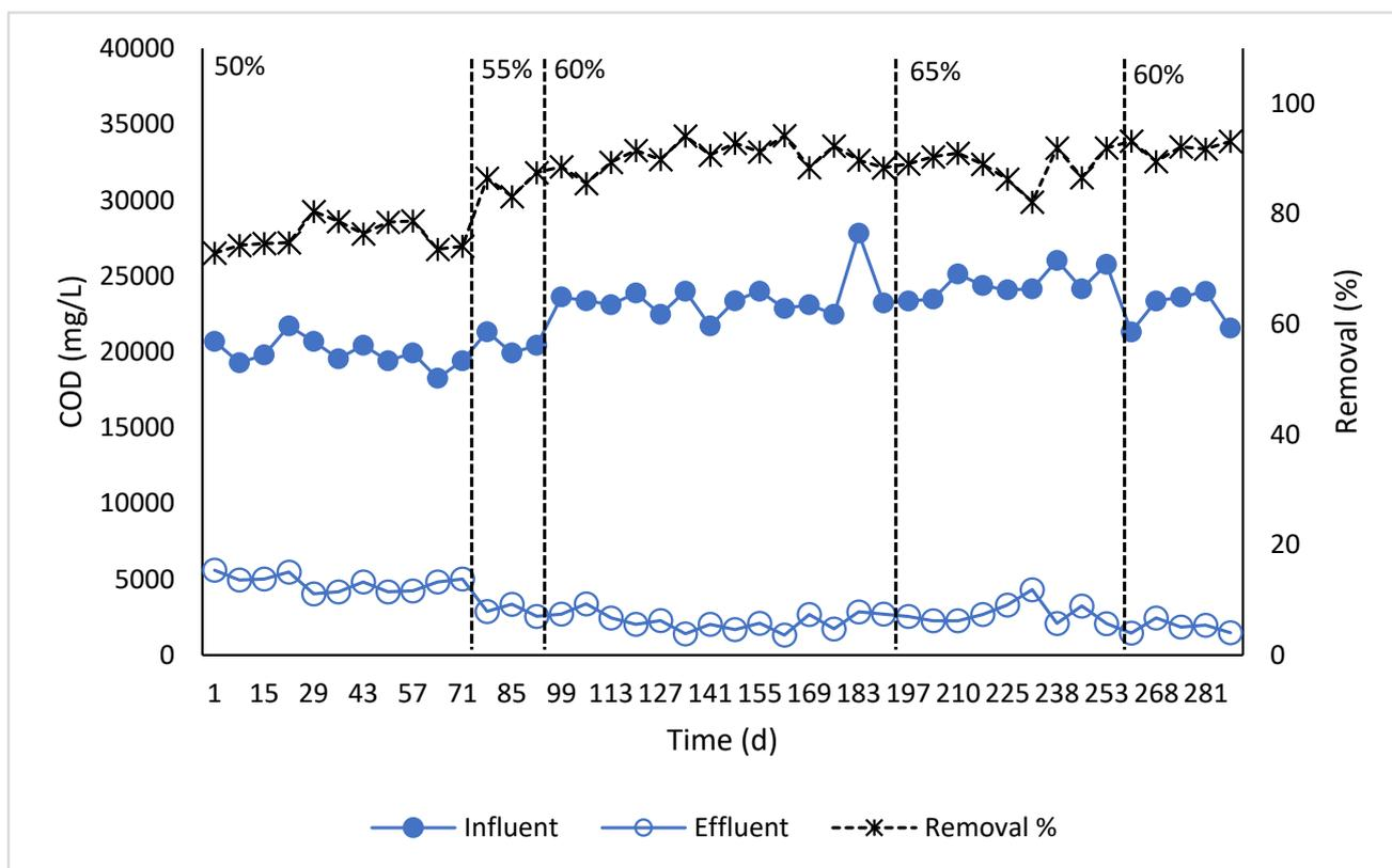
Figure 7. Behavior of COD with increasing initial vinasse concentration from 50% to 60%.
