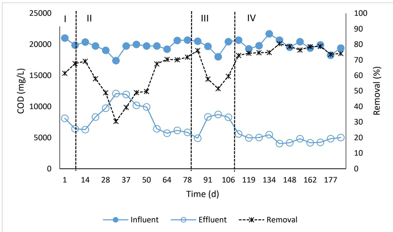
**Figure 5.** COD behavior during carbon/nitrogen (C/N) ratio adjustment: Stage I—Addition of 2.4 g/L NH<sub>4</sub>Cl, Stage II—Two doses of 2.4 g/L NH<sub>4</sub>Cl in the first 4 cycles, Stage III—1.3 g/L CO(NH<sub>2</sub>)<sub>2</sub> in the first 3 cycles, Stage IV—Addition of 1.1 g/L NH<sub>4</sub>Cl in all cycles.
