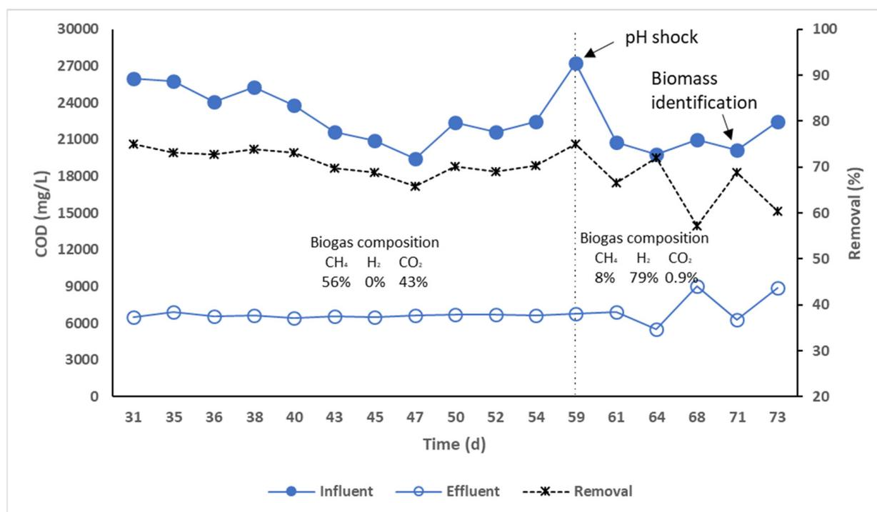
**Figure 1.** COD behavior during the transition from a methanogenic microbiota to an acidogenic one within an A-SBR.
