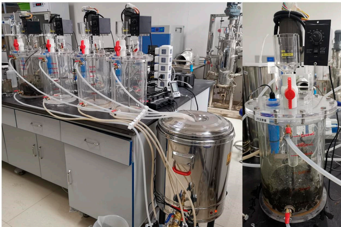
Figure 2. Each of the CSTR reactors used in the experiment was equipped with its own dedicated control and detection system.
