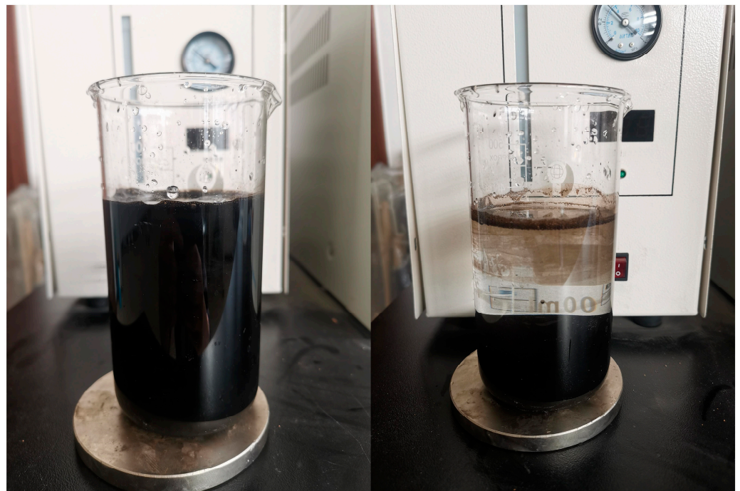
Figure 4. The magnetic separation effect of \text{Fe}_3\text{O}_4\text{@BC} (after completely mixing the nanoparticles with water, placing a magnet at the bottom, and allowing it to stand for 5 min to observe the effect).
