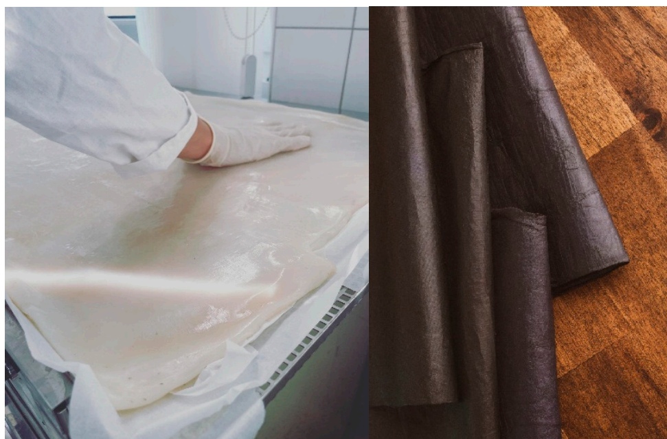
Figure 2. Wet BC pellicle (left side) and BC-based vegan leather (right side). Photo Credits: Smoby, Hungary [36].
