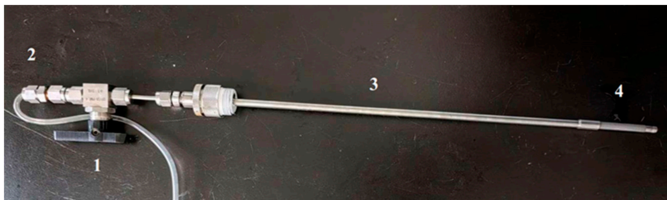
1: Switch valve. 2: Gas interface. 3: Gas guide metal pipe. 4: Metal membrane tube.
