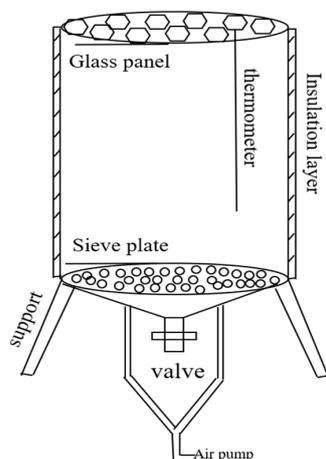
**Figure 1.** Composting unit diagram.
