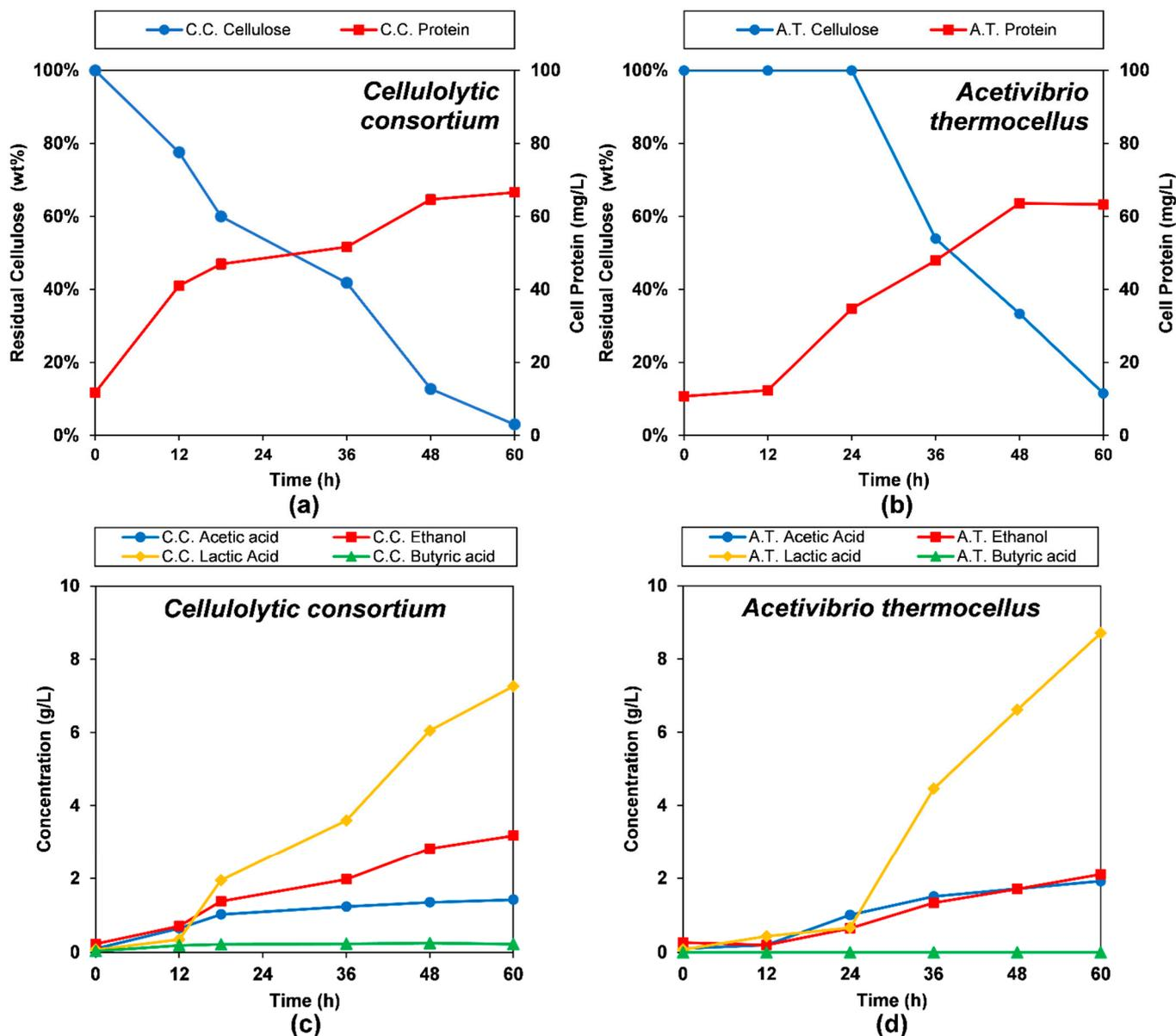
**Figure 3.** Conversion of cellulose to end-products in 2 L bioreactors with 20 g/L cellulose by a cellulolytic consortium (C.C.) and *A. thermocellus* (A.T.): (a) cellulose utilization and Bradford protein for C.C. cultures; (b) cellulose utilization and Bradford protein for A.T. cultures; (c) end-products for C.C. cultures; (d) end-products for A.T. cultures.
