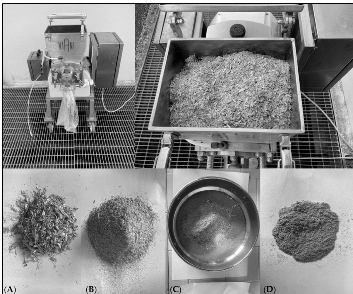
Figure S2. Cereal mill used in the preparation of the agro-waste and different stages of preparation of the agro-waste. Original emmer and oat chaff agro-waste (A) ; agro-waste after milling (B) , sieving through 40 mesh (C) , sieved, ready to use material (D) .
