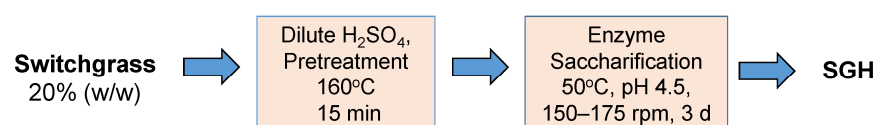
Scheme 1. Process diagram showing dilute sulfuric acid pretreatment of switchgrass followed by enzyme saccharification to switchgrass hydrolysate (SGH).
