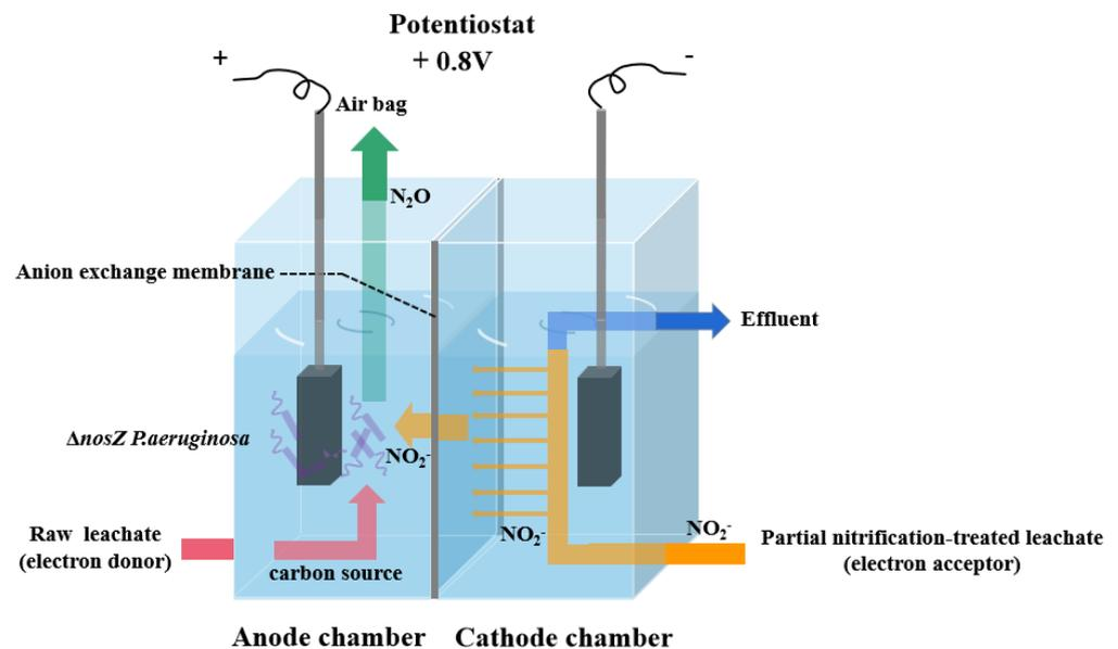
**Figure 1.** Schematic diagram of the  $\Delta nosZ$  *P. aeruginosa*/MEC system.
