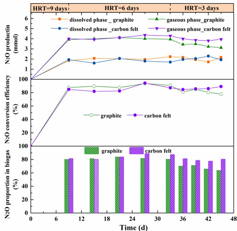
**Figure 3.** Nitrous oxide conversion of  $\Delta nosZ$  *P. aeruginosa*/MEC systems with carbon felt electrodes and graphite electrodes. (a)  $N_2O$  production; (b)  $N_2O$  conversion efficiency; (c)  $N_2O$  proportion in biogas. Error bars represent standard deviations of triplicate measurements.
