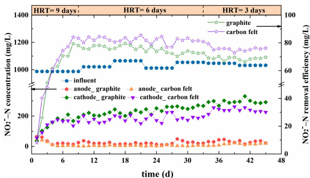
**Figure 2.** Nitrite removal of  $\Delta nosZ$  *P. aeruginosa*/MEC systems with carbon felt electrodes and graphite electrodes.
