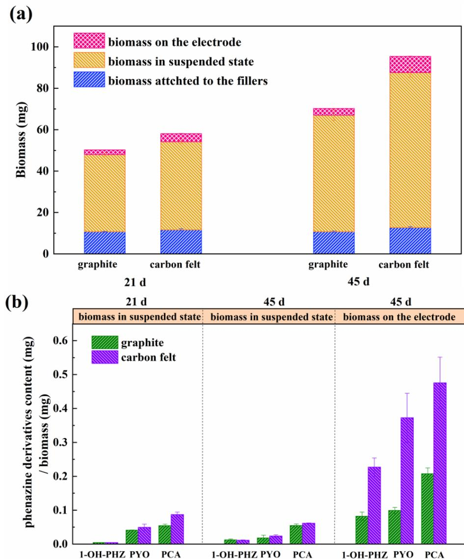
**Figure 5.** Biomass and the opportunity of touching phenazine derivatives per unit of biomass in the  $\Delta nosZ P. aeruginosa$ /MEC systems with carbon felt electrodes and graphite electrodes on day 21 and 45. (a) Biomass; (b) phenazine derivative content/biomass. Error bars represent standard deviations of triplicate measurements.
