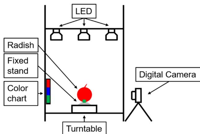
**Figure 1.** Schematic diagram of the experimental device.
