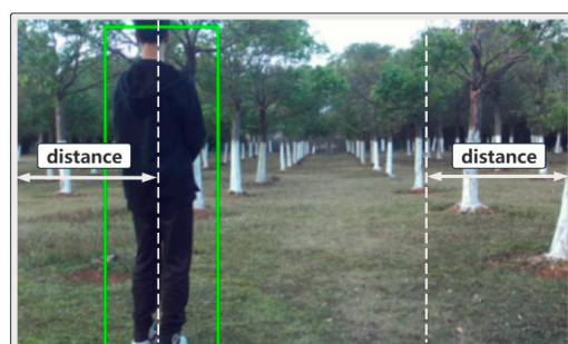
Figure 5. The trigger region of the KCF algorithm. The distance is denoted as dis in this paper.
