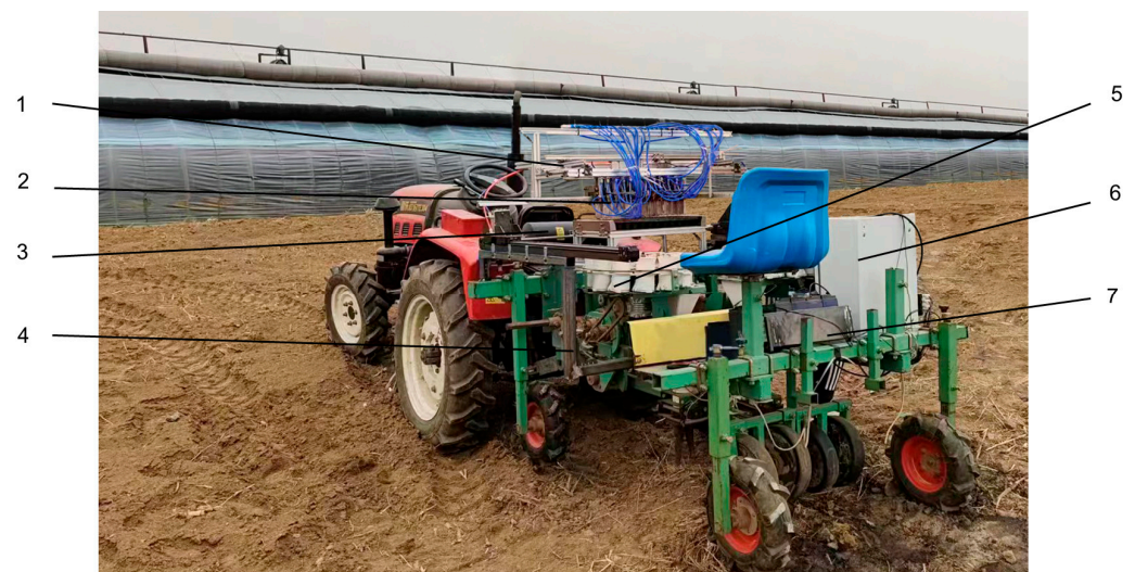
Figure 14. Transplanting experiment. 1. Transplanting arm; 2. Transplanting manipulator; 3. Air compressor; 4. Planting device; 5. Seedling separation device; 6. Power distribution and PLC control system; 7. Battery. Traction double-row automatic transplanter needs two operators. One person needs to drive the tractor, and the other needs to alter the seedling tray.
