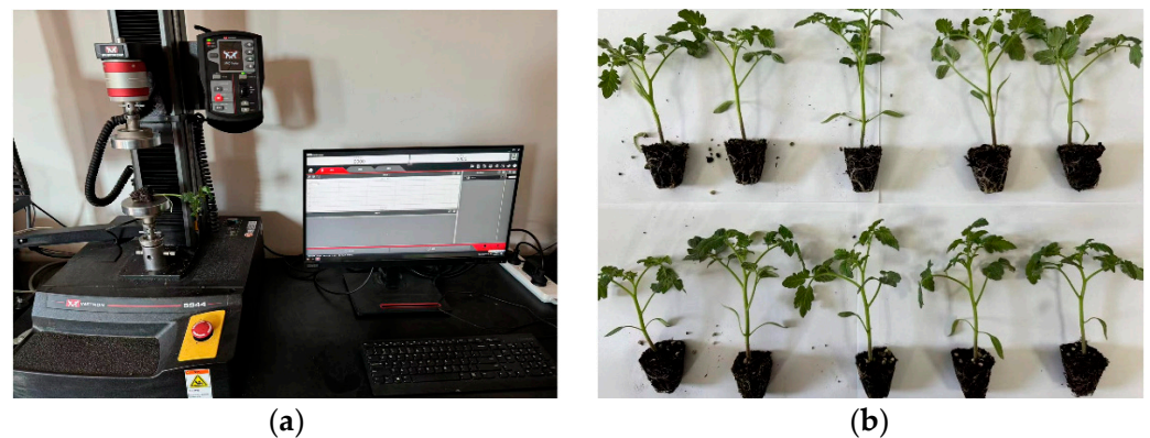
Figure 6. Shear force experiment. (a) Shear force test platform; (b) experimental seedlings.
