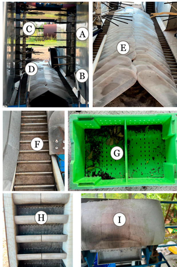
Figure 1. Graphic illustration of sampling sites of over-the-row harvesters. Note: the top loader has sites A to I, but the bottom loader only has sites A to G. A: upper side wall; B: lower side wall; C: upper beat bars; D: lower beat bars; E: catcher plate; F: horizontal conveyor belt; G: berry lug; H: vertical conveyor belt; I: filling flap in Georgia or upper conveyor in Oregon.
