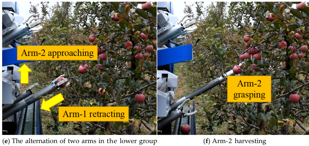
Figure 2. An example of the alternation for multi-arm harvesting robots.
