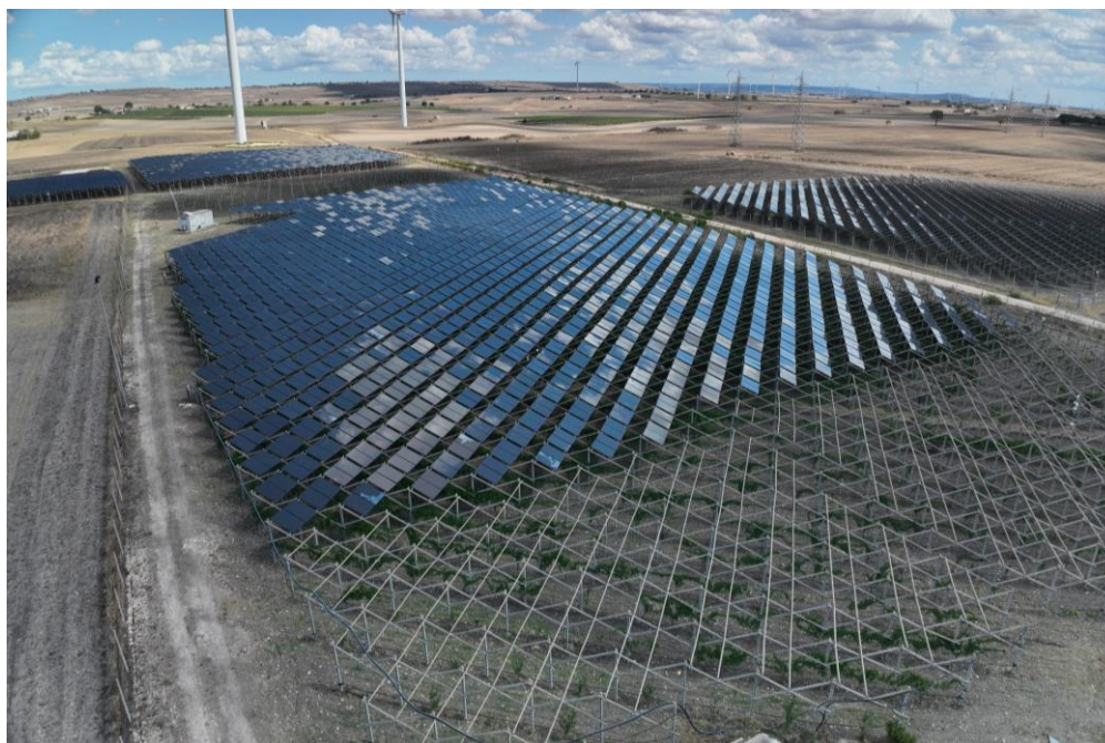
Figure 1. View of the agrivoltaic vineyard, with the AV treatment above and full-sun exposure below.
