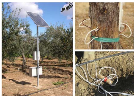
Figure 7. System used by the author to measure sap flow in olive trees with the compensation heat pulse method. It consisted of a solar panel and weather-proof boxes for the electronics (upper box) and battery (lower box) (left). Also shown are sap flow probes inserted into the trunk and a main root of olive trees (right).
