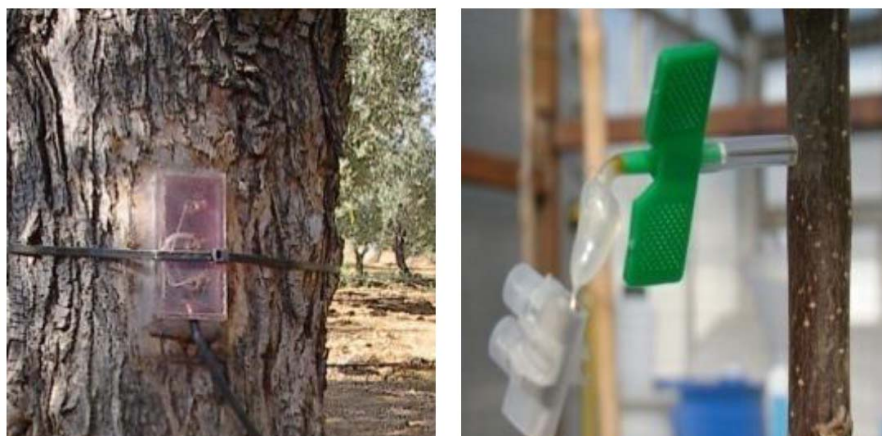
Figure 10. A TDR probe installed in the trunk of an olive tree for volumetric water content-related measurements ( left ). The photo was taken during a joint experiment of the author with Dr. Arie Nadler (Institute of Soil, Water, and Environmental Sciences, ARO, Rishon LeZion, Israel), who manufactured the probe. A probe for electric potential-related measurements in the stem of a young fruit-tree ( right ), manufactured by Dr. Luis Gurovich (Department of Fruit Science, Pontificia Universidad Católica de Chile, Santiago, Chile).
