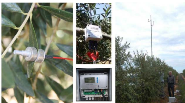
Figure 9. Installing the ZIM system in the orchard mentioned in Figures 1 and 6, with the help of Ulrich Zimmermann (in the photo on the right). ZIM probes (left) were connected to a radio transmitter (central up), which sent the collected records to a data logger (central down) located in a weather-proof box at the base of a pool with two aerials (right), one for the radio signals and the other for sending the data from the data logger, via GPRS, to a server.
