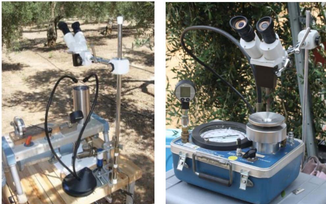
Figure 3. Scholander chambers for measuring approximate water potential of plant tissue. A model by Soilmoisture Equipment Corp., Santa Barbara, CA (USA), implemented with a binocular stereo microscope and a cold light illuminator (left), and a model by PMS Instrument Company, Albany, OR (USA), implemented with a binocular stereo microscope and a digital manometer (right).
