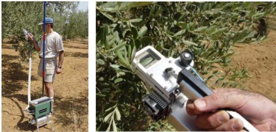
Figure 2. Measuring leaf gas exchange in olive with a photosynthesis system (model LI-6400, LI-COR, Lincoln NE, USA), implemented with a tube to sample the air from above the tree canopies and a deposit for mixing the reference air before going through the analyzer ( left ). Detail of the chamber used for measurements under the prevailing light conditions ( right ).
