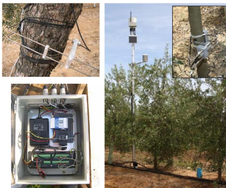
Figure 8. Two different systems for the automatic recording and data transmission of trunk diameter variations. The system on the left consists of LVDT (linear variable differential transformer) dendrometers connected to a Campbell CR1000 data logger (Logan, UT, USA). On the right, a Verdtech station with Plantsens radial dendrometers (Verdtech un Nuevo Campo S.A., Lepe, Spain) is shown, along with a C-Probe (AquaSpy, Inc., San Diego, CA, USA) for the measurement of the soil volumetric water content, two Rain-O-Matic tipping-bucket gauges (Pronamic Co. Ltd, Sikeborg, Denmark), one to record the water supplied by the irrigation system and the other for the precipitation amounts; a combined sensor of temperature and humidity of the air (Vaisala Oyj, Helsinki, Finland) and an addWAVEA733GSM remote telemetry unit (Adcaon Telemetry, Klosterneuburg, Austria).
