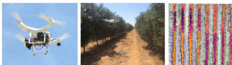
Figure 6. Images corresponding to the work by Egea et al. [65] in which a thermal infrared (TIR) camera (Tau 2 324, FLIR Systems, Inc., Wilsonville, OR, USA) was mounted on a multirotor RPAS (Remote Piloted Aerial System) model Phantom 2 (SZ DJI Technology Co., Ltd., Shenzhen, China) for thermal imagery acquisition in a high hedgerow olive orchard with 1667 trees per ha ( left ). Several 0.4\text{ m} \times 0.5\text{ m} black plastic panels were used as a hot reference ( central ). Images were taken at 20 m above ground and at solar noon of two fully irrigated plots (purple and blue colors) and two deficit-irrigated plots (yellow and orange colors) ( right ).
