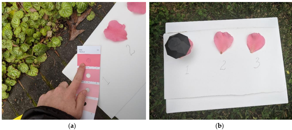
Figure 3. Example of measuring camellia petal color using: (a) the Royal Horticultural Society (RHS) Colour Chart [10], and (b) the Nix TM Pro color sensor [11].
