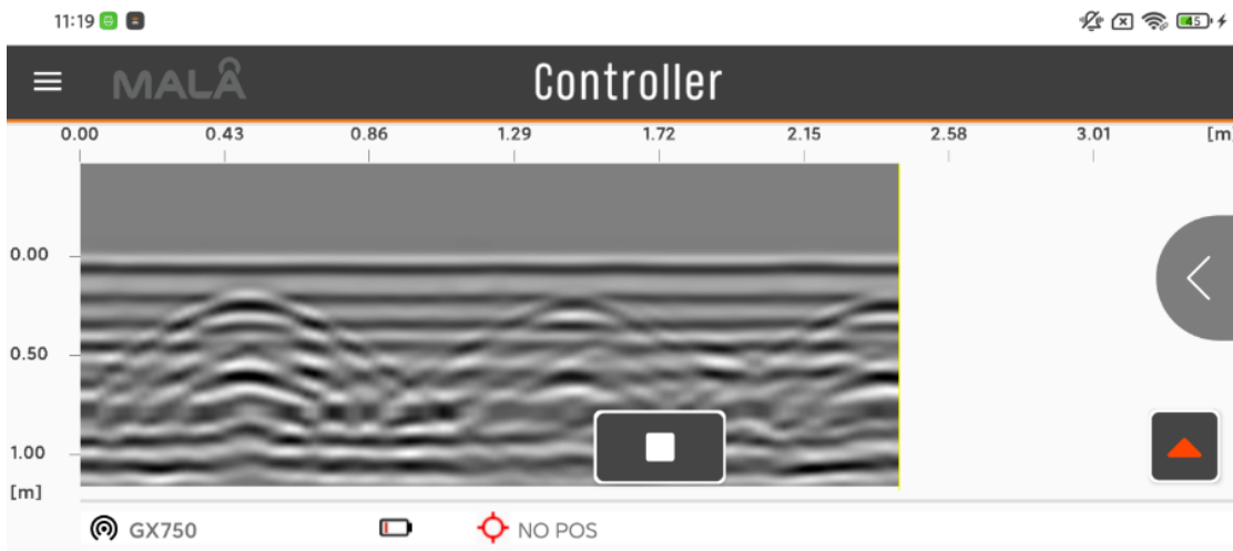
(d) The resulting image recorded by the ground-penetrating radar above the third steel bar.
