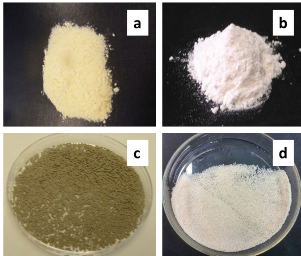
Figure 6. Examples of physical aspect from different solid formulates: (a) freeze-drying WP, (b) spray-drying SP, (c) fluidized bed drying WG and (d) fluidized bed spray-drying WG.
