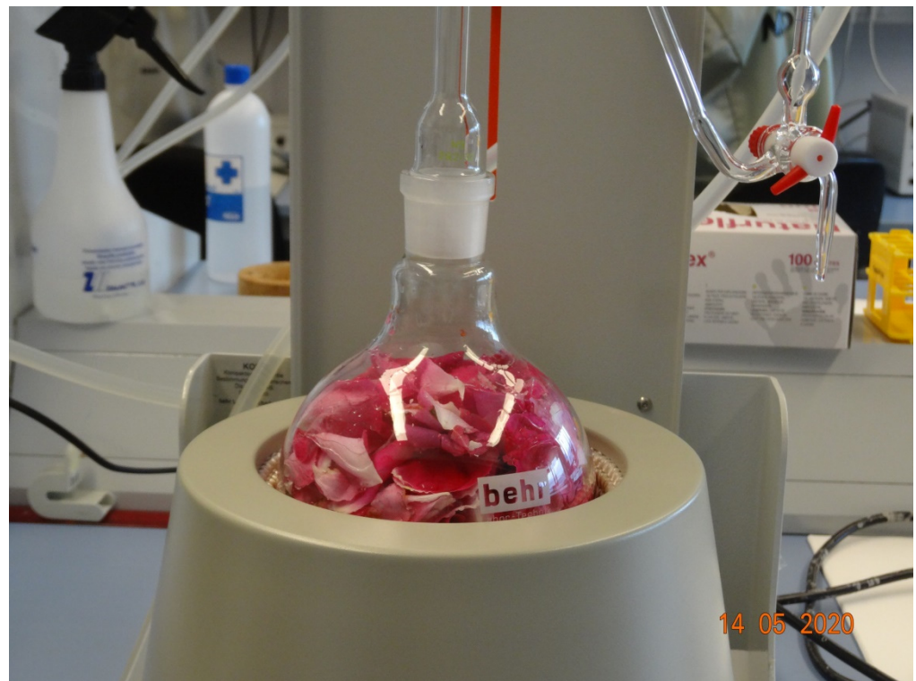
Figure 2. Hydrodistillation apparatus with flask charged with petals.
