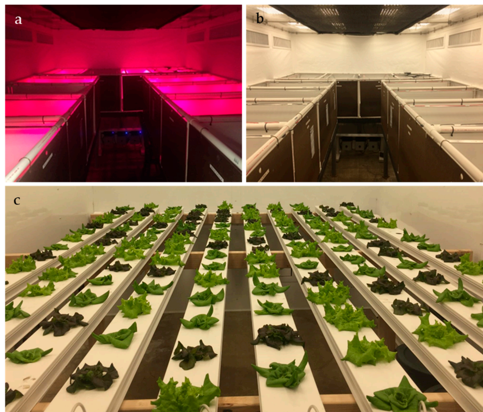
Figure 2. Experimental grow configuration of lettuce seedling growth chamber with (a) only far-red LEDs and (b) with base white LEDs. (c) Nutrient film technique chamber with white LEDs.
