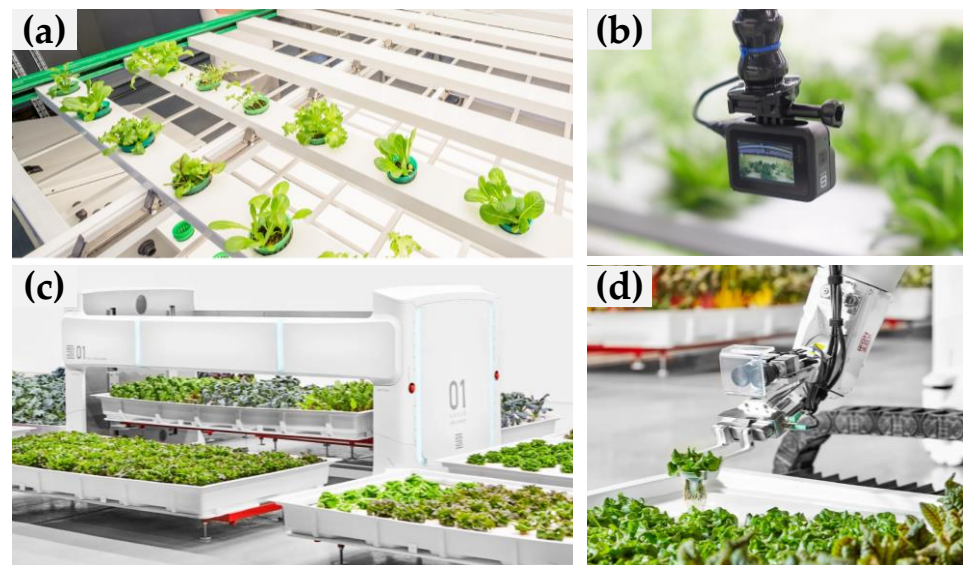
Figure 9. Unmanned operation in vertical farming: (a) automatic conveyor belt (adapted from [133]); (b) control video camera on a rack (adapted from [133]); (c) 1000-pound robot named Angus (adapted from [136]); and (d) Iron Ox’s robotic arm for harvesting (adapted from [136]).
