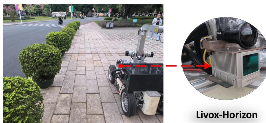
Figure 1. Data acquisition equipment and scene. In order to ensure that the LIDAR can acquire the height of the hedge from bottom to top, the installation height of the LIDAR in this study was about 0.8 m. In other working scenarios, the height of the LIDAR needs to be adjusted according to the height of the hedge.
