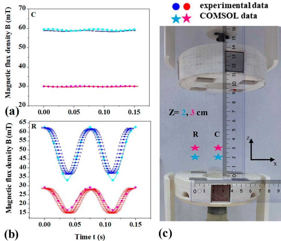
**Figure 9.** Experimental validation of the time dependency of the magnetic flux density B (a) at the center of the disk (C) and (b) at 3 cm distance from the center of the disk (R). Blue and red data correspond to the (c) experimental measurements 2 and 3 cm above the disk, while cyan and magenta mark the corresponding COMSOL-simulated AMFs for the respective coordinates.
