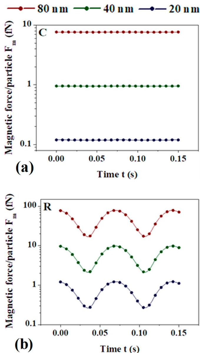
**Figure 7.** Time evolution of the exerted magnetic forces per ferromagnetic particle of varying size. The curves are at the plane with  $z = 0$  cm, meaning two millimeters above the bottom array. C and R shown in (a,b), respectively, denote the characteristic points in those planes, the coordinates of which were reported in the previous section.
