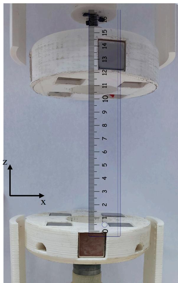
**Figure 2.** Schematic illustration of the z-levels and the arbitrarily set zero value. For this paper, the plane that is 2 mm (typical width of a petri dish bottom) above the top surface of the Halbach array that has been colored blue corresponds to  $z = 0$  cm. Furthermore,  $z = 1$  cm indicates a 1 cm distance from the top surface,  $z = 2$  cm correlates to a 2 cm distance, etc.
