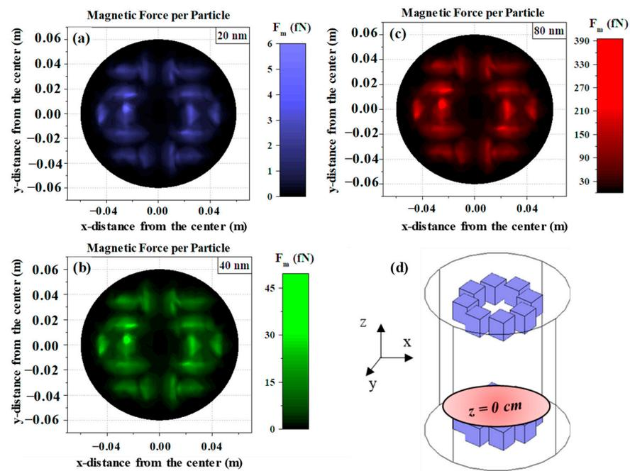
**Figure 4.** Magnetic forces exerted on a single ferromagnetic particle of (a) 20 nm, (b) 40 nm, and (c) 80 nm size. The axes express the vertical and horizontal distance from the center of the plane similarly to Figure 3. (d) All three contour plots are the product of a numerical analysis in the plane that is 2 mm above the top surface of the magnets of the bottom configuration.
