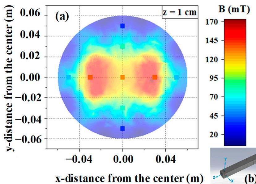
**Figure 8.** Experimental validation of the static magnetic flux density at a plane 1 cm above the bottom array. (a) The Hall magnetometer utilized to collect experimental data. (b) The nine non-transparent squares correspond to the measurements registered with the aid of the Hall magnetometer. These points are plotted against the computationally derived magnetic field strength at the corresponding  $z$ -level.
