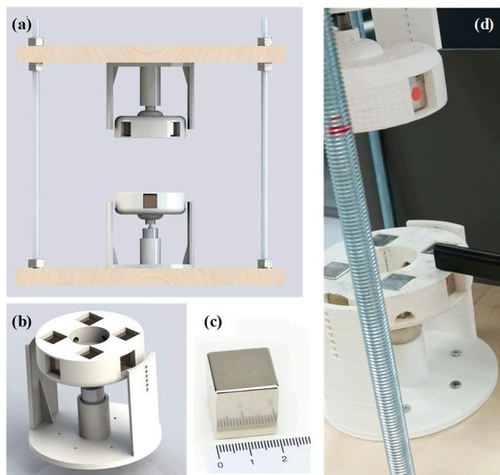
**Figure 1.** The experimental setup of the designing platform and in real life. (a) Complete composition of the disk screwed on wooden platforms and connected with metal screw rods. (b) The model of one disk in the CAD environment. (c) Permanent magnet placed in the cubic host slots. (d) Photograph taken of the setup, where all the parts have been assembled.
