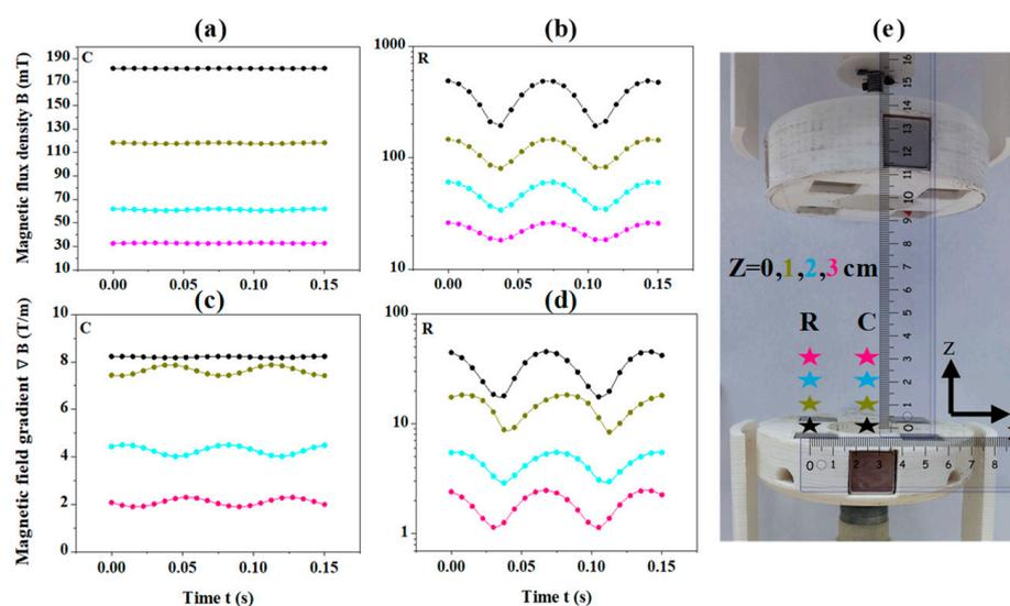
**Figure 6.** Time evolution of the magnetic flux density (a,b) and the magnetic field gradient (c,d). The plots denoted as C (a,c) correspond to simulations at the center of the disk, whereas plots denoted as R (b,d) describe B at the periphery of the conceived aperture cylinder as depicted in (e). The colors black, olive, light blue, and magenta correspond to the heights above the bottom array with  $z = 0, 1, 2,$  and  $3$  cm, respectively.
