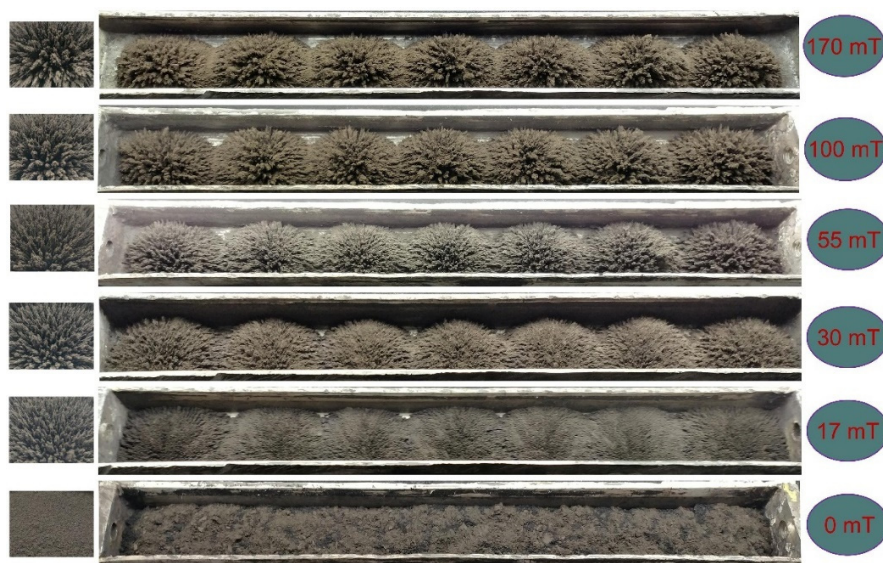
Figure 7. Photograph showing CoFe 2 O 4 @Ag 2 O nanocomposites arranged in a photochemical reaction with different strengths of magnetic field. Reprinted from Jiang et al. [119] with permission from Elsevier.
