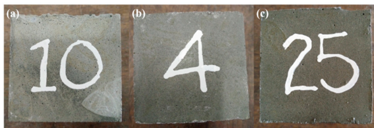
Figure 2. Physical appearances of unexposed fly ash geopolymers with (a) 0%, (b) 2% and (c) 4% of silica fume.
