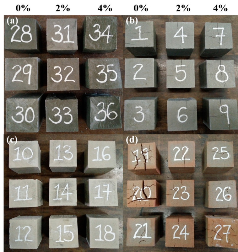
Figure 3. Physical appearance of fly ash geopolymers with varying silica fume content: (a) unexposed; (b) 200 °C; (c) 600 °C; and (d) 1000 °C.
