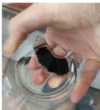
**Figure 1.** Magnetic adsorbent during the washing stage, showing its attraction to a stationary magnet.
