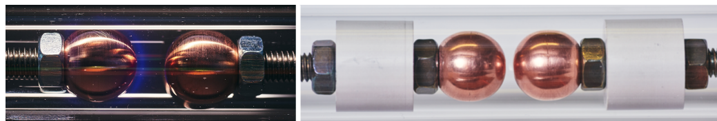
Figure 5. (Left) Cylinder and electrode set A, (Right) cylinder and electrode set B, with additional supporting alignment. The electrodes are manufactured from copper.
