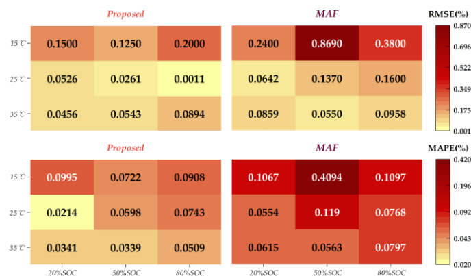
Figure 10. A comparison of the RMSE and MAPE of the two methods in nine test cases.
