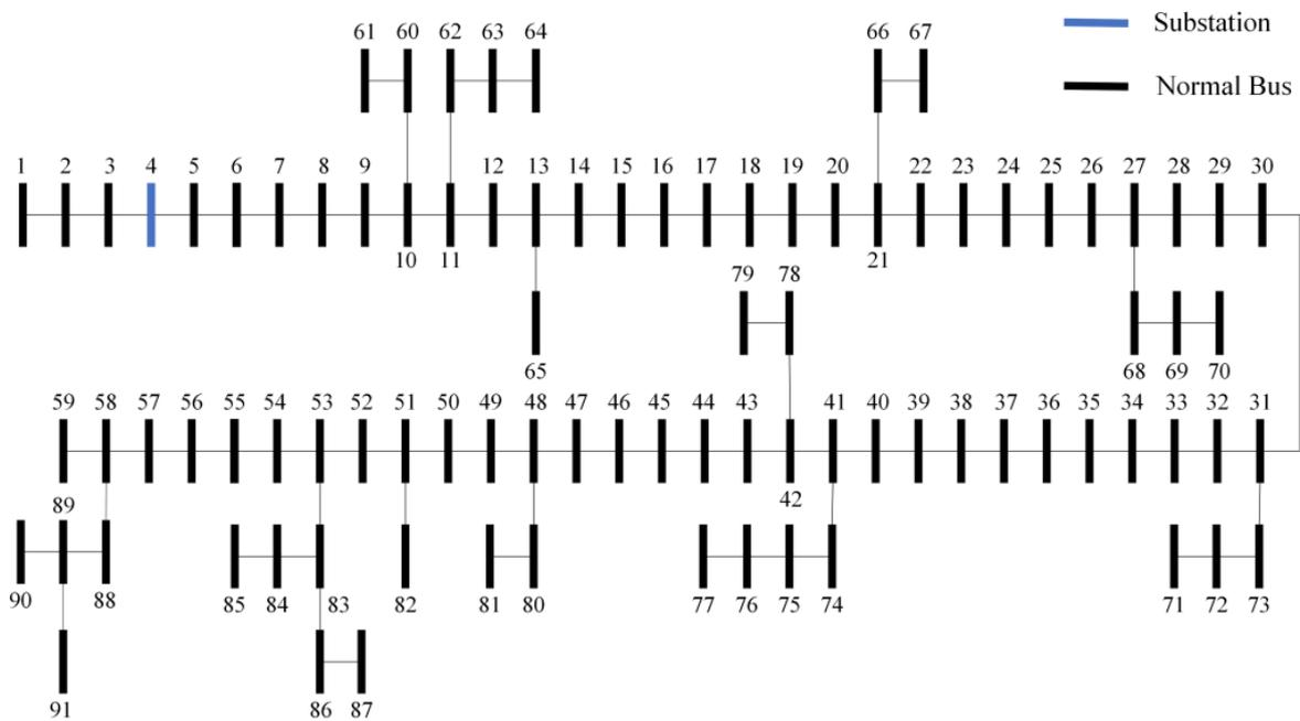
Figure 2. Single-line diagram of the PLA10 distribution network.
