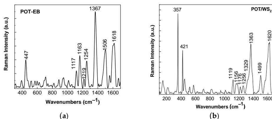
**Figure 7.** The Raman spectra of POT-EB (a) and the POT/WS<sub>2</sub> composite (b), with a TMD concentration of 20 wt.%, synthesized by ICP of OT.
