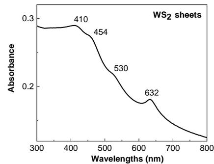
**Figure 5.** UV-VIS spectrum of WS<sub>2</sub> sheets resulting from mechanical exfoliation at 900 rpm, followed by ultrasonication in DMF.
