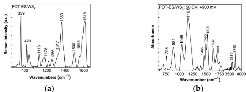
**Figure 11.** Raman spectrum (a) and FTIR spectrum (b) of the POT-ES/WS<sub>2</sub> composite synthesized by ECP on the Pt electrode surface after recording 50 cyclic voltammograms.
