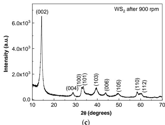
**Figure 3.** (a) XRD diagrams of WS<sub>2</sub> nanoparticles before and after grinding at 150, 300, 600, and 900 rpm. (b,c) X-ray diagrams of WS<sub>2</sub> nanoparticles before and after 900 rpm.
