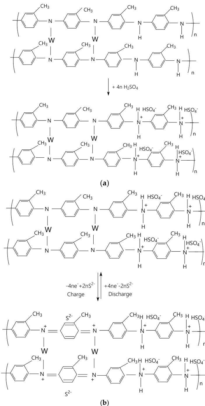
**Scheme 4.** Reactions during discharge and charge processes in SC cell containing POT-ES/WS<sub>2</sub> composite as EAM: (a) the reaction of the POT-LB/WS<sub>2</sub> composite with H<sub>2</sub>SO<sub>4</sub> (Equation (1)) and (b) charge/discharge processes of the POT-LS/WS<sub>2</sub> composite (Equation (2)).
