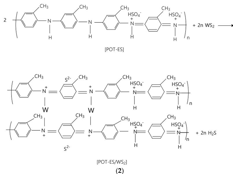
**Scheme 2.** The mechanism of EC synthesis of the POT/WS<sub>2</sub> composite: (1) oxidation reaction of POT-LS with the generation of POT-ES; (2) chemical interaction of POT-ES with WS<sub>2</sub>.
