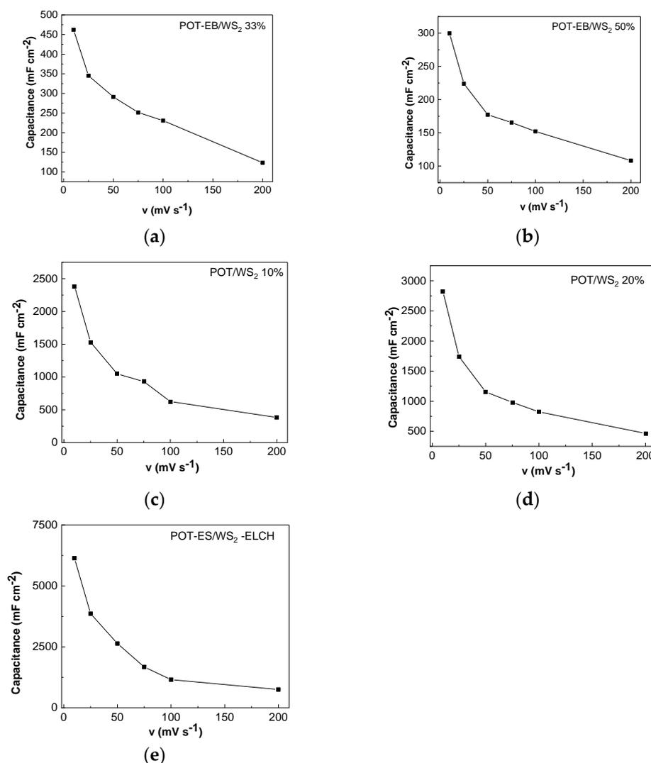
**Figure 16.** The dependence of capacitance vs. potential scan rate of electrodes based on the POT-EB/WS<sub>2</sub> composites resulting from SSI with WS<sub>2</sub> concentrations equal to 33 wt.% (a) and 50 wt.% (b); the POT-EB/WS<sub>2</sub> composites synthesized by ICP with WS<sub>2</sub> concentrations equal to 10 wt.% (c) and 20 wt.% (d); and the POT-ES/WS<sub>2</sub> composite synthesized by the ECP method (e).
