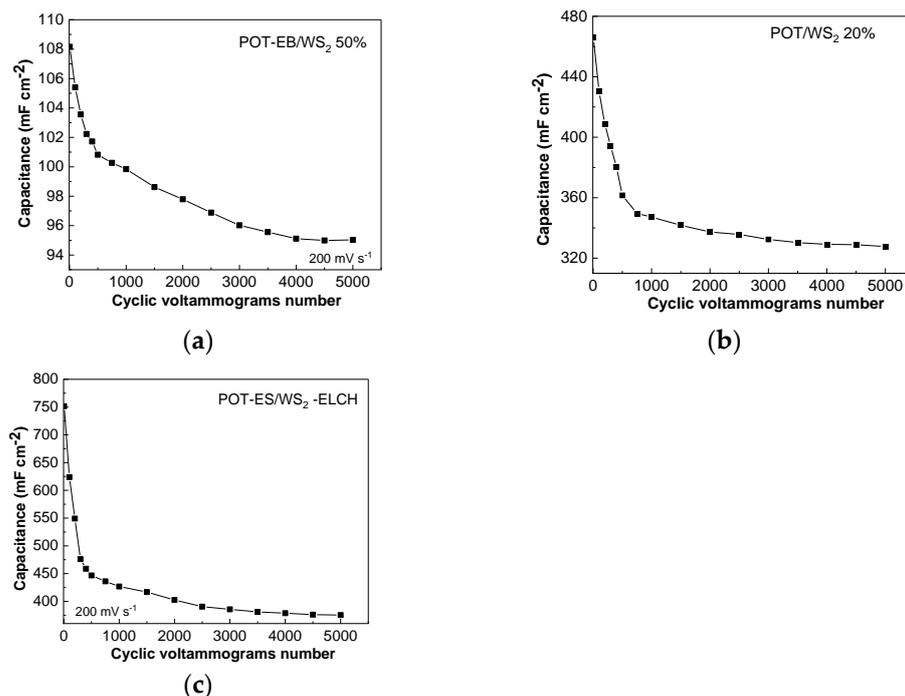
**Figure 17.** The variation in capacitance vs. number of cyclic voltammograms recorded at  $200 \text{ mV s}^{-1}$  of electrodes based on (a) the POT-EB/ $\text{WS}_2$  composite prepared by the SSI method, when the  $\text{WS}_2$  concentration in composite mass was 50 wt.%; (b) the POT/ $\text{WS}_2$  composite, synthesized by ICP (the  $\text{WS}_2$  concentration in the composite mass was 20 wt.%); and (c) the POT-ES/ $\text{WS}_2$  composite, synthesized by the ECP method.
