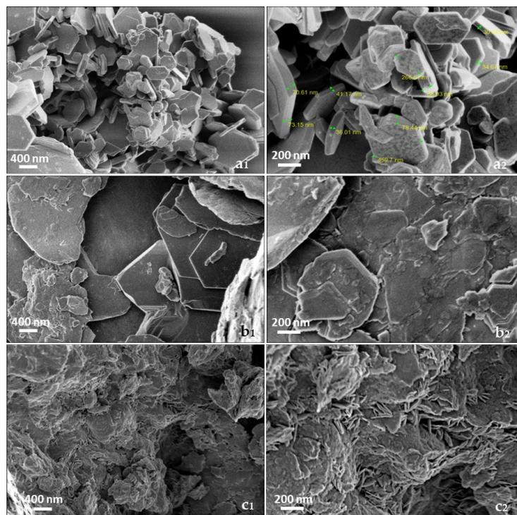
**Figure 1.** SEM images of WS<sub>2</sub> flakes (a<sub>1</sub>,a<sub>2</sub>); the WS<sub>2</sub> nanosheets resulting from grinding flakes for one hour at 600 rpm (b<sub>1</sub>,b<sub>2</sub>) and 900 rpm (c<sub>1</sub>,c<sub>2</sub>).
