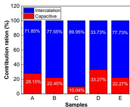
**Figure 15.** Contribution ratio between capacitive and diffusion processes of POT-EB/WS<sub>2</sub> composites with WS<sub>2</sub> concentrations of 33 wt.% (sample A) and 50 wt.% (sample B), the POT/WS<sub>2</sub> composites synthesized by the ICP method (WS<sub>2</sub> concentration in composite mass is 10 wt.% (sample C) and 20 wt.% (sample D)), and the POT-ES/WS<sub>2</sub> composite synthesized by the ECP method (sample E).
