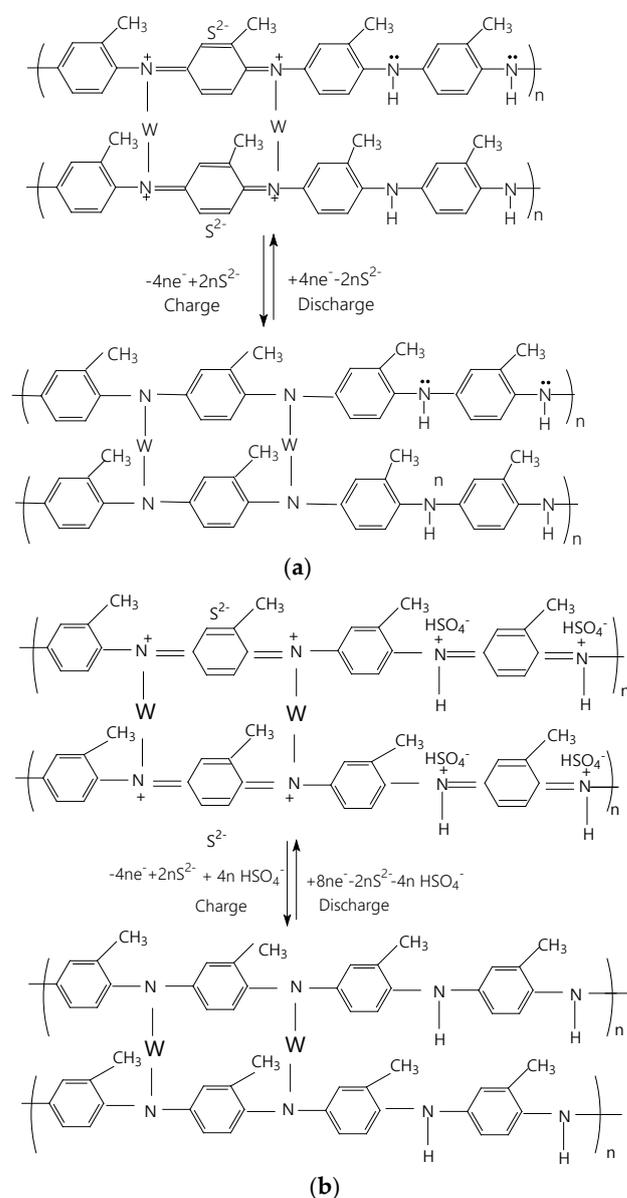
**Scheme 3.** The reactions at the electrolyte/electrode interface of the electrodes containing the POT/WS<sub>2</sub> composites synthesized by ICP (a) and the POT-ES/WS<sub>2</sub> composite synthesized by ECP (b).
