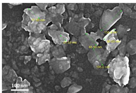
**Figure 2.** SEM image of WS<sub>2</sub> sheets.
