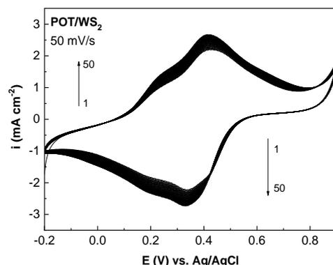
**Figure 10.** The first 50 cyclic voltammograms of ECP of OT in a solution of  $\text{H}_2\text{SO}_4$  and  $\text{WS}_2$  sheets, recorded at a potential scan rate of 50 mV/s.
