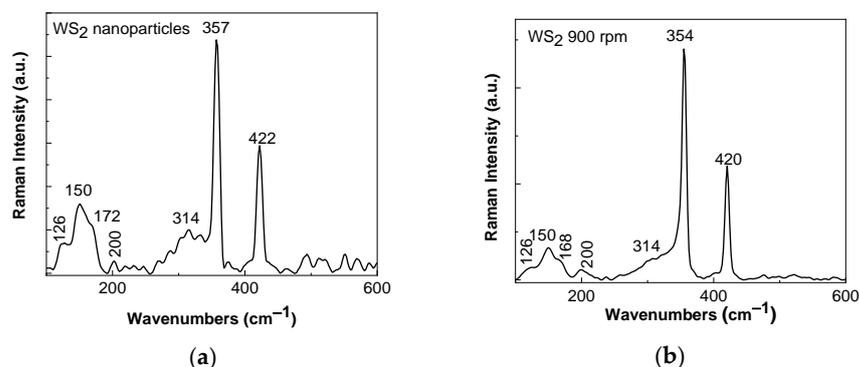
**Figure 4.** The Raman spectra of WS<sub>2</sub> NPs before (a) and after grinding exfoliation at 900 rpm (b).
